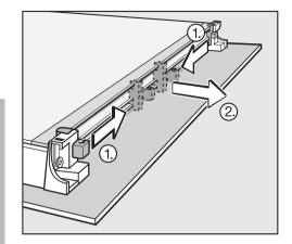
Push the spacers towards the centre of the door and then pull them off. If they are difficult to remove lift the middle pane up a little. The spacers should then be easier to move.
